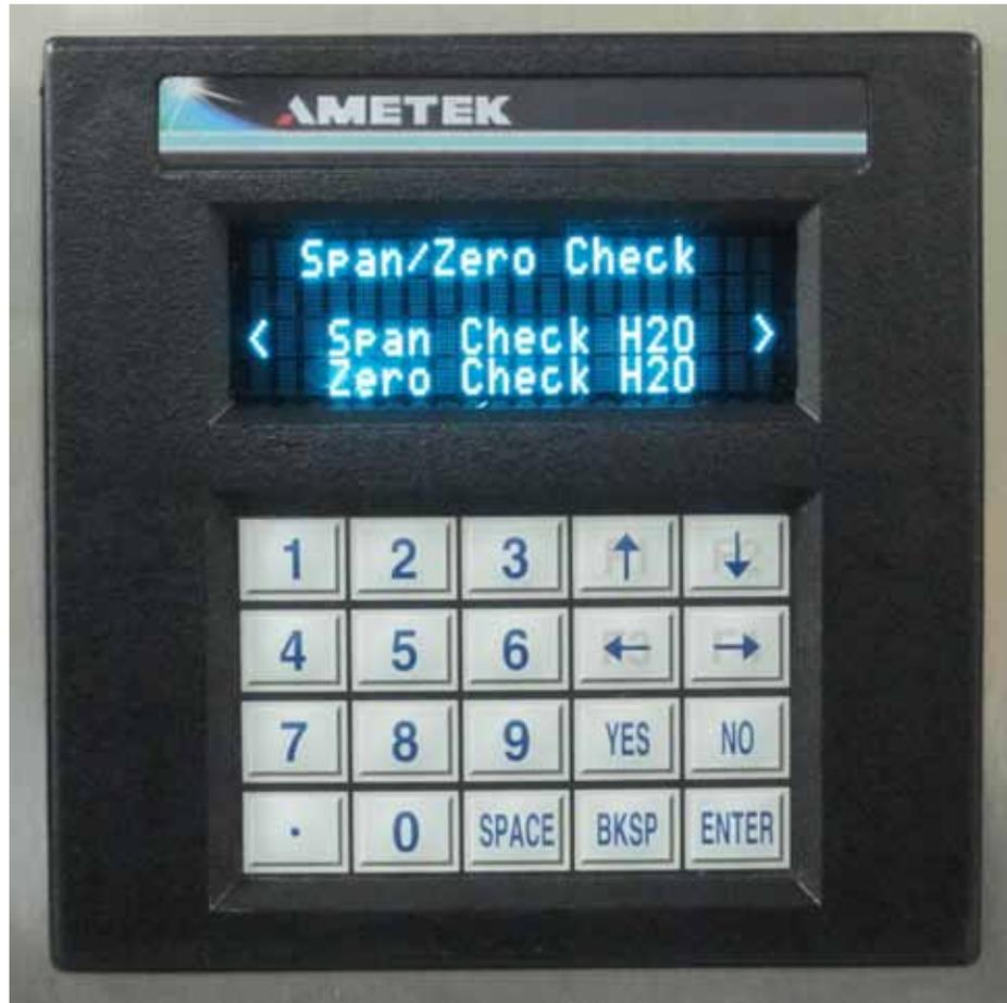
To perform a Span Check, scroll to that selection and press ENTER. The following screen will be displayed (for H2O in this example):
