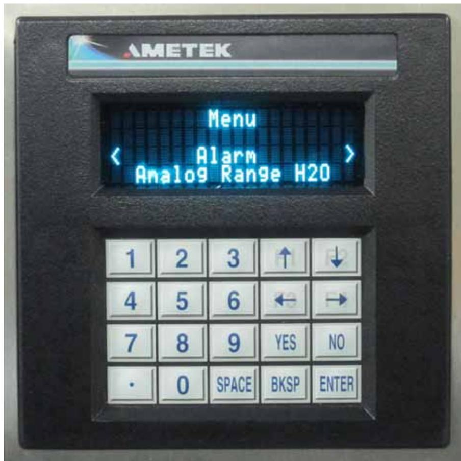
Scroll down to the “Span/Zero Check” menu selection using the down-arrow key:
