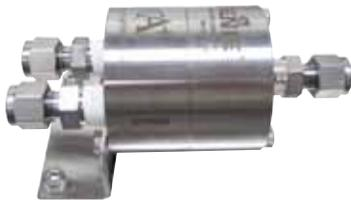
The separator inside the sample section removes entrained liquids and particulates from the gas before it passes through the sample cell. For this reason, the bypass or drain valve is left OPEN to allow the residue to exit the analyzer. Ensure that the valve is turned slightly to the OPEN position.
