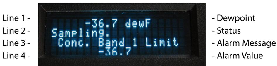
**Figure 4-1b. Display for alarm condition.**
