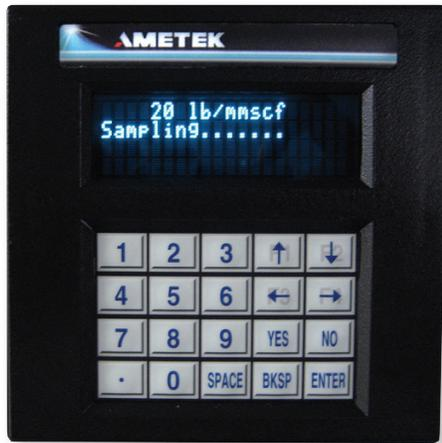
The Model 5100 Analyzer keypad (Figure 3-11) is used to access menus, sub-menus and system values, and to set-up analyzer parameters.
