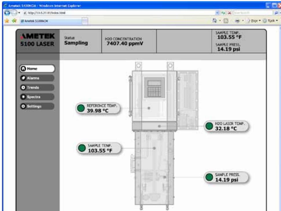
Figure 5-2. Model 5100 analyzer web interface Home screen.
